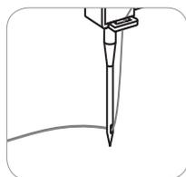
6. If you want to thread the needle manually, thread it from front to back. Pull about 6-8 inches of thread to the back beyond the needle eye. Alternatively, you can use the automatic needle threader to thread the eye of the needle. (see page 16)
